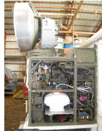
Fire control radar adapted for biological use
